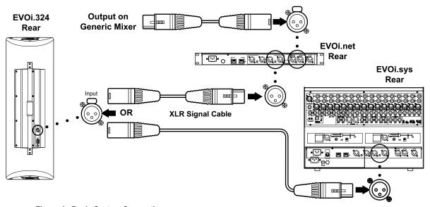
Figure 4 - Basic System Connections
